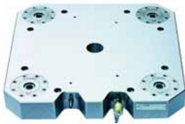
Fast closing clamp plate with 4 pcs of flushed SPEEDY assembly round 1000.
