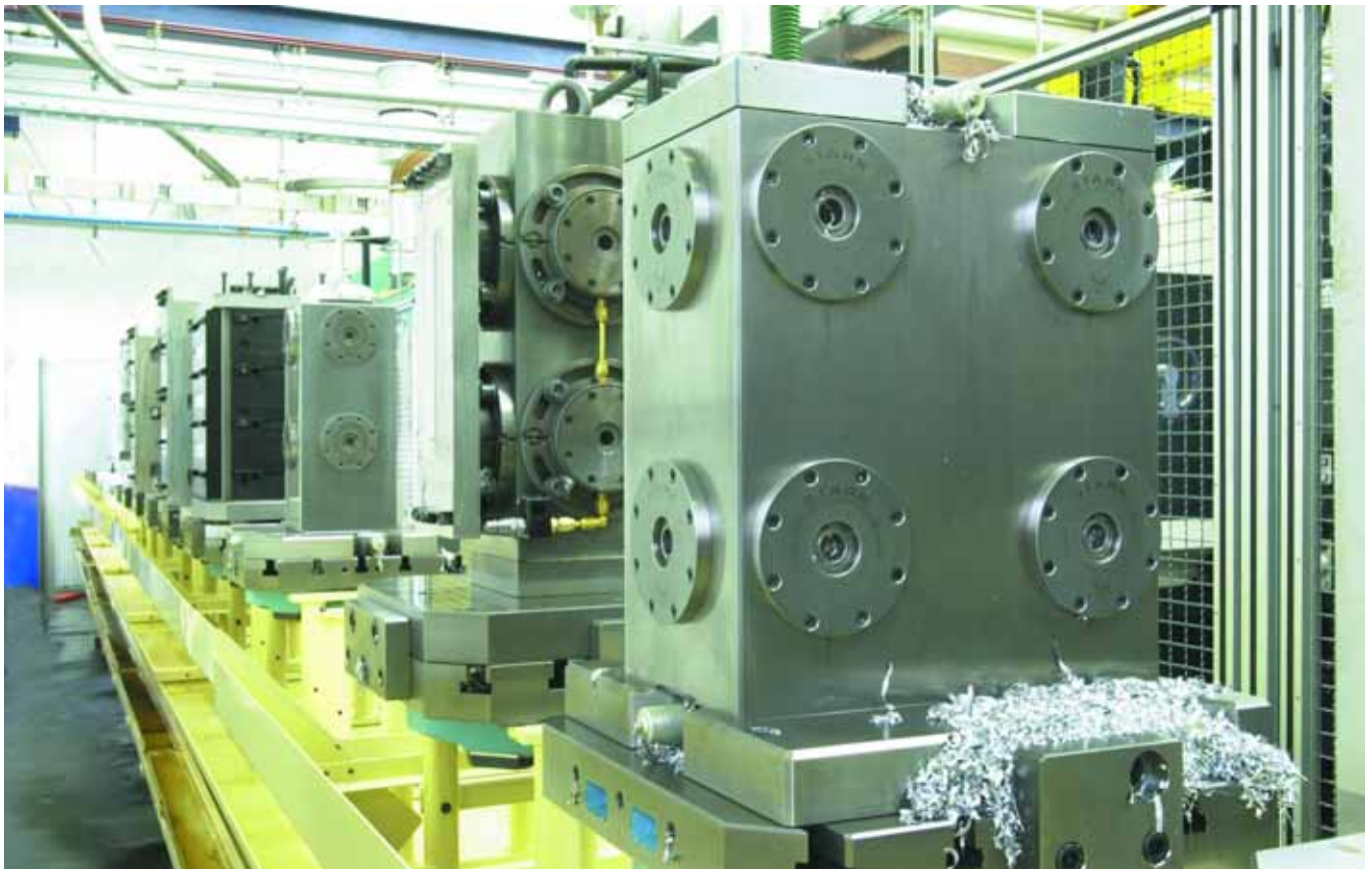
Pallet station with mounting towers, SPEEDY 1000 tubular set up and SPEEDY 1000 assembly
